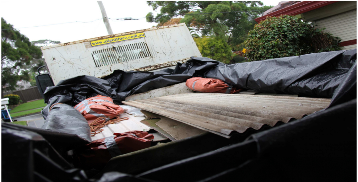
Figure 1. Asbestos cement sheet collected during the free asbestos collection trial.
